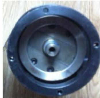
5. Cup folding parts is controlled by three separate cams, and each folding clip can be adjusted by itself.
