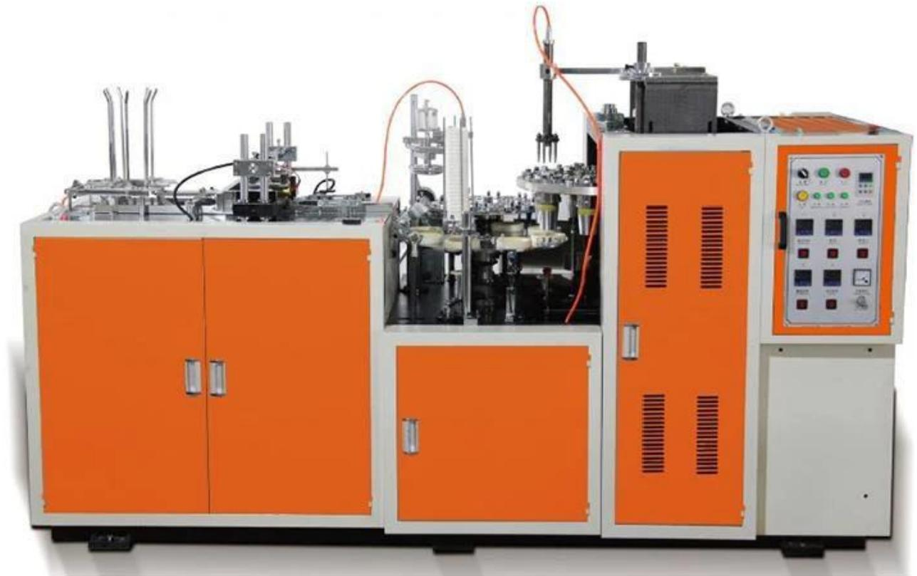
ZB-D paper cup machine is improved based on the open cam system. This machine runs a whole procedure of paper-feeding, cup-fan-wall sealing, oiling, and bottom punching, heating, rolling, rimming, rounding and tripping. It is idea equipment for producing drinking cups, market cups, coffee cups, advertising cups, etc. It is widely used for hot drink and beverage.
