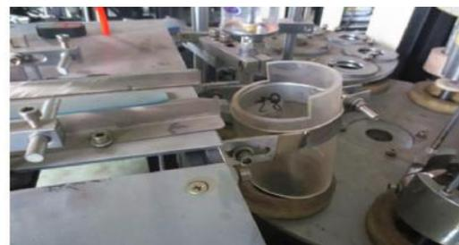
7. Change the  $\text{Ø}25$  normal steel shaft to  $\text{Ø}30$  imported steel shaft to be strengthened, longer life and more stable.
